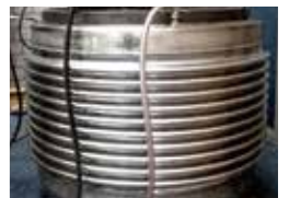
Specimen after 6023 load cycles
