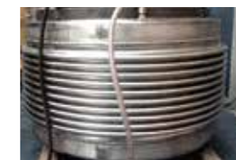
Specimen after 1560 load cycles
